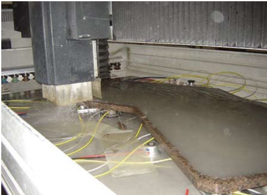
A Park Destiny dual-spindle CNC Stonecenter is also used in the slab fabrication process.
