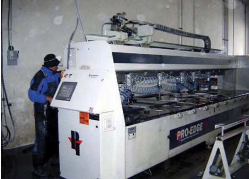
The 22,000-square-foot facility in Sacramento is also equipped with a Park Pro Edge III automatic edge machine.
