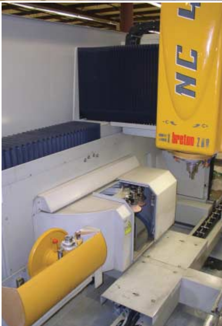
The machine features automatic tool changing of up to 27 different tools, and it can also use one of two blades as needed.
