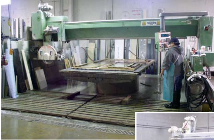
A Pedrini bridge saw was the first piece of equipment purchased by the company.
