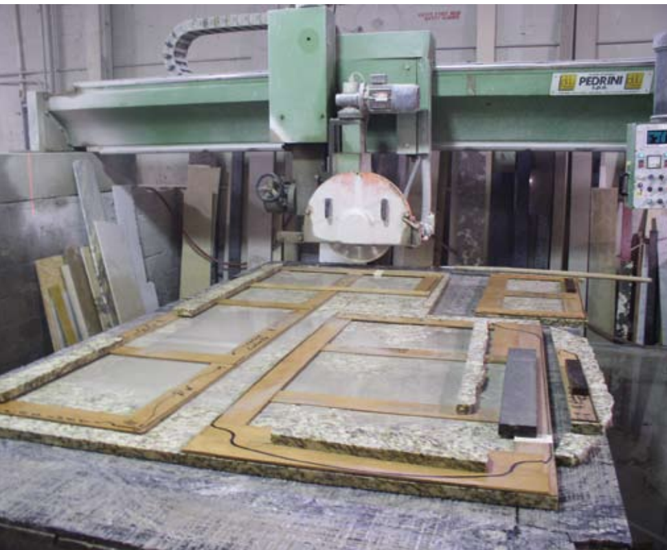
The templates are also physically laid out on the slabs during the cutting process.
