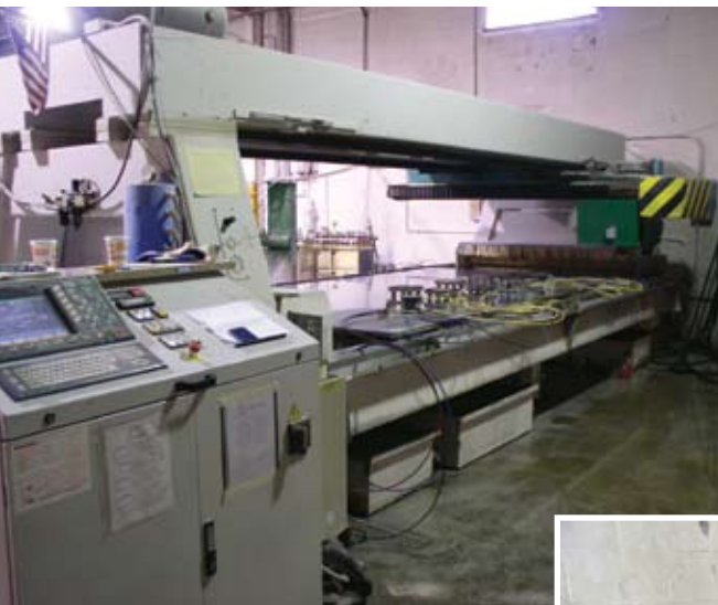
After material is cut to size, more intricate stone processing is done on an Intermac Master Stone 4000 CNC stoneworking center, which was purchased from AGM.
