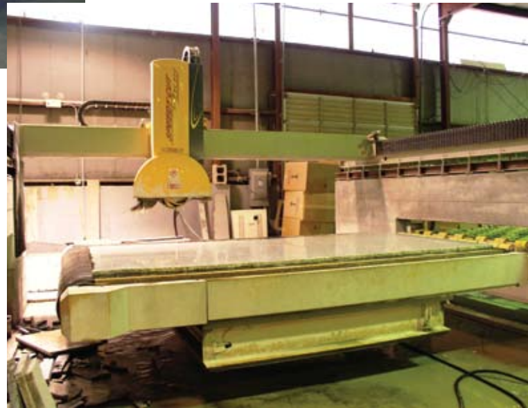
The Speedy Cut saw can cut up to 800 square feet in eight hours and a full slab in 20 to 25 minutes.
