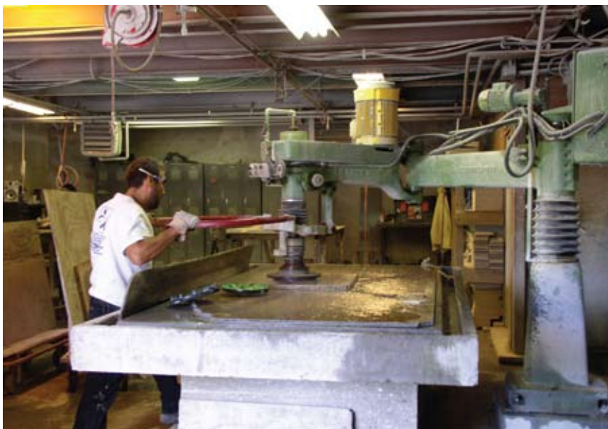
A F. Zambon radial arm polisher allows for different finishes to be given to stone pieces.
