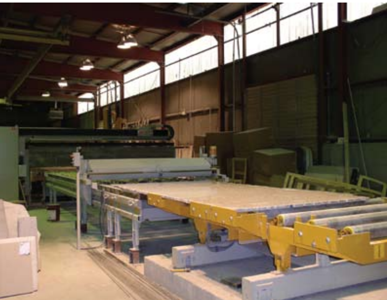
Once on the conveyor, slabs are moved to the Breton Speedy Cut fully automatic bridge saw for processing.
