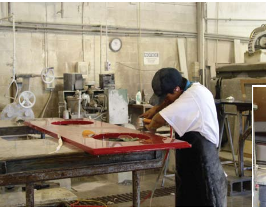
Hand tools are used to put finishing touches on the edges of natural stone and engineered quartz countertops.
