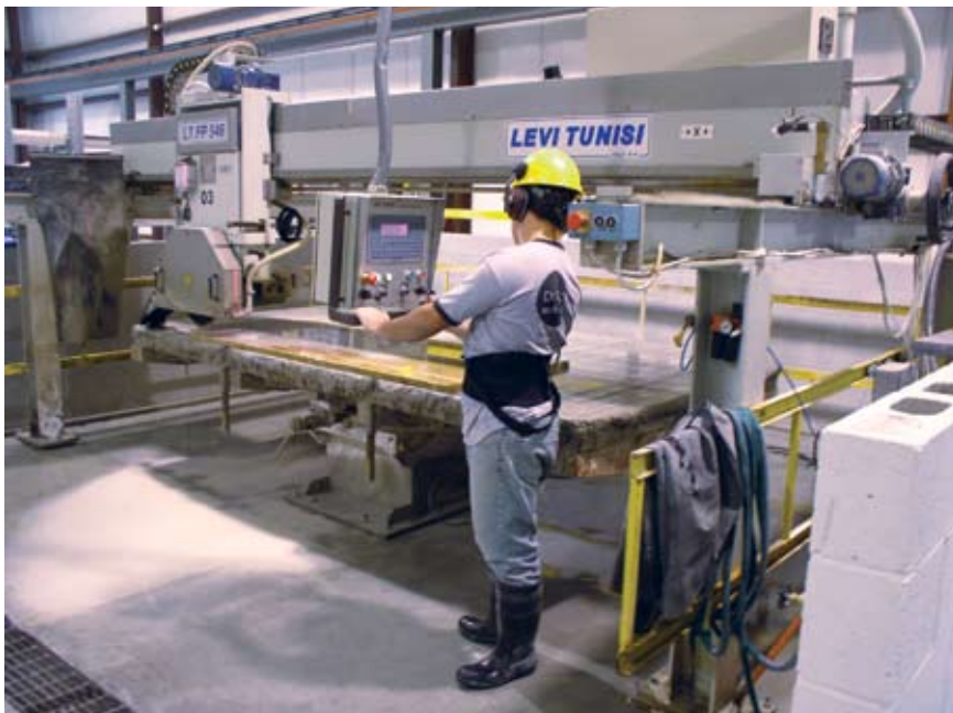
The Millbury location operates a programmable Levi Tunisi bridge saw, which it purchased from International Machine Corp. of Holbrook, NY.
