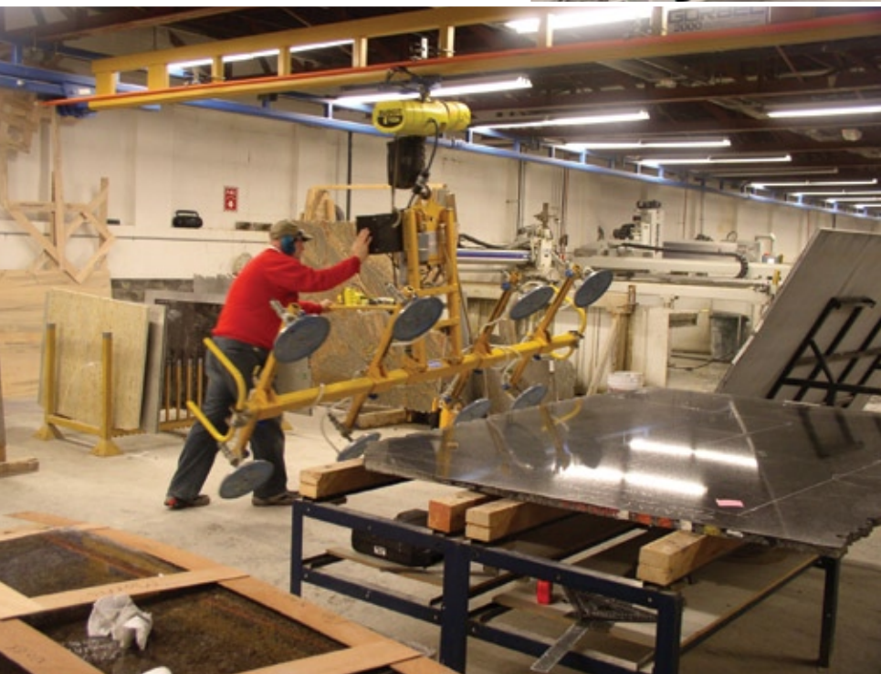
Slabs are maneuvered using a Gorbel 2000 overhead crane system from Mass Crane and Hoist, which is equipped with an eight-pad vacuum lifter from Anver.
