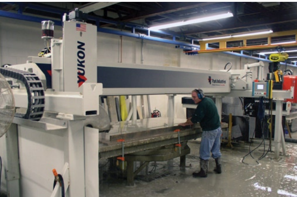
A Yukon bridge saw from Park is among the other recent technology investments.
