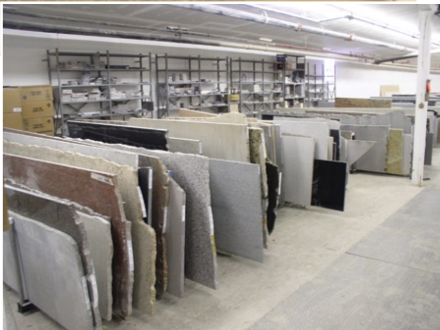
Slabs are stored on racks supplied by GranQuartz, and in addition to storing unprocessed slabs, the company also has racks and a dedicated area for storing its stone remnants, each of which are inventoried in the company’s system.
