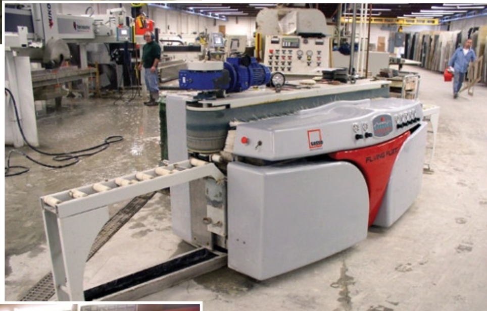
A Sasso Flying Flat edging machine from U.S. Granite Machinery is used for processing backsplashes.
