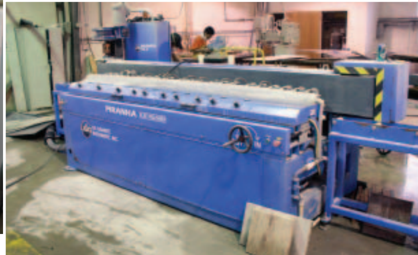
Straight polishing is completed with a Piranha edging machine from U.S. Granite Machinery.
