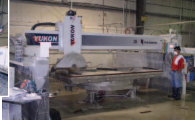
Slab cutting is also completed with a Park Industries Yukon bridge saw.
