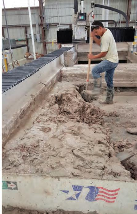
**Figure 2** — CNC collection trays and sawjet tables that can hold thousands of gallons of water can also hold large amounts of potentially dangerous sludge.
